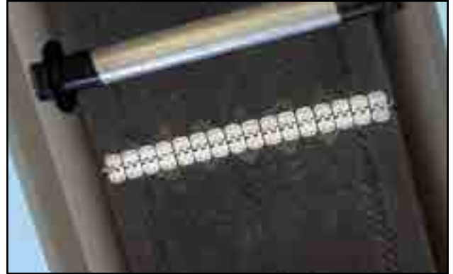
Fig 52 - Conveyor belt lacing
