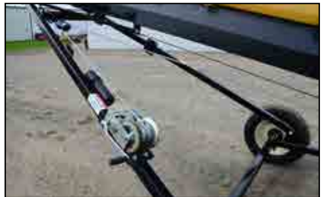
Fig 18 - Tube Lift Winch
