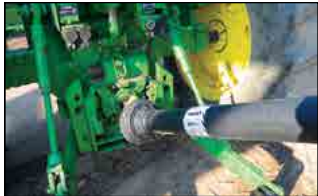
Fig 26 - PTO attached to tractor
