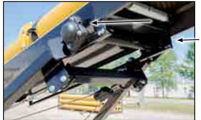
Fig 45 - Upper lift bearings
