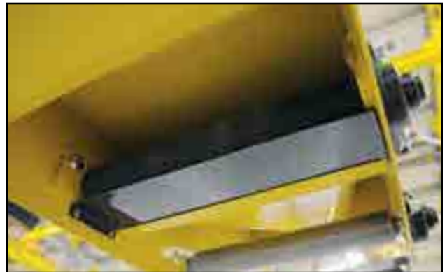
Fig 54 - Containment plate in place
