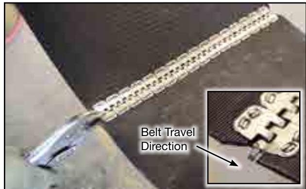
Fig 59 - Crimp lacing and taper belt corner
