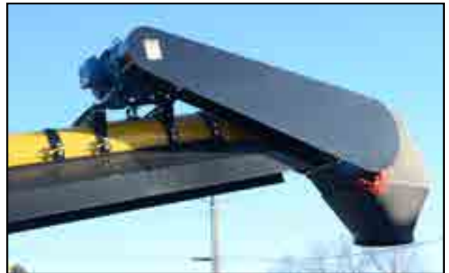
Fig 33 - Top-end electric drive
