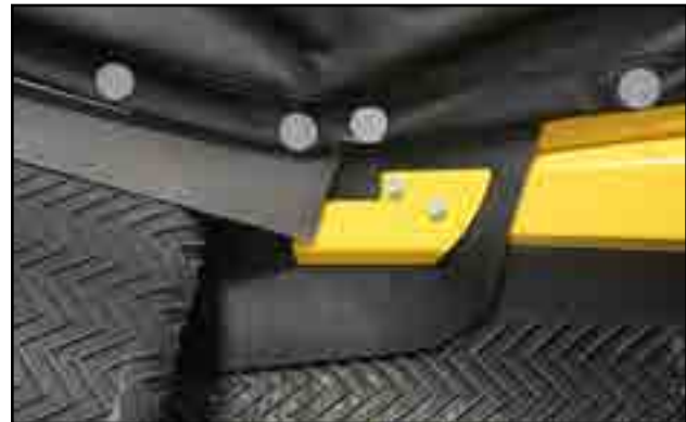
Fig 69 - Fasten flashing clamp
